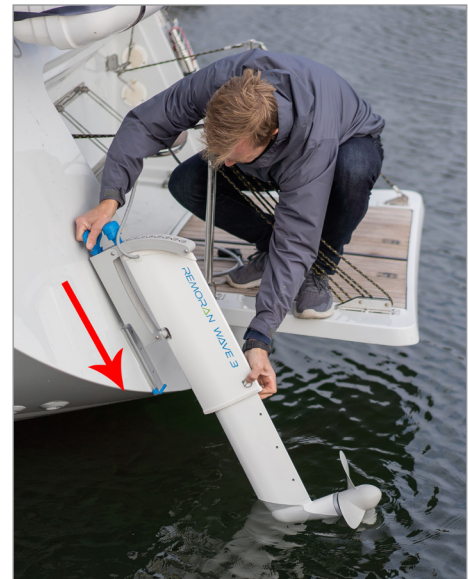
[Figure 27] Place the frame of the outboard unit to the top of the rail and slide it down along the rail.
