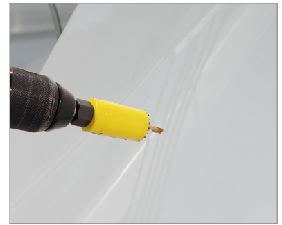
[Figure 13] Drill a 22 mm hole to the boat transom for the feedthrough of cables
