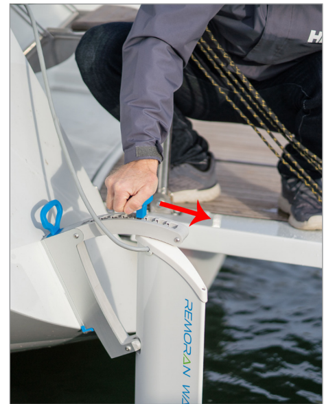
[Figure 29] Adjust the outboard unit to a right angle in relation to the water surface
