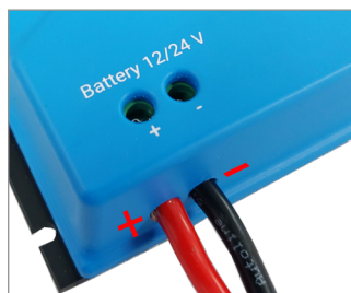
[Figure 17] Carefully connect the charging wires to the appropriate apertures with the + and - wires in their appropriate locations.
