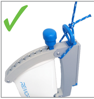
[Figure 23] Using a safety rope with the hydrogenerator
