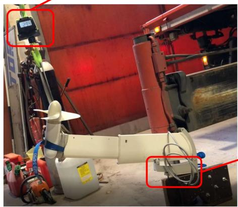
Overall mechanical endurance of the outboard generator unit exceeds 294 kgs, which was the limit of test setup as the screws used to attach the rail to a block of plywood came loose. The outboard unit itself suffered no damages and remained fully operational after the testing. The only event was the triggering of the mechanical fuse as intended.
