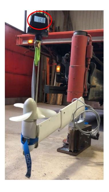
Limit of mechanical fuse – 168 kg Test was performed with a crane and the outboard unit fully extended. Actual fuse threshold on a partially extended unit is higher.
