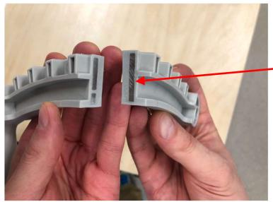
The critical plastic parts are molded over a stainless steel core and the actual plastic is reinforced with fibers to ensure high mechanical durability and strenght.
