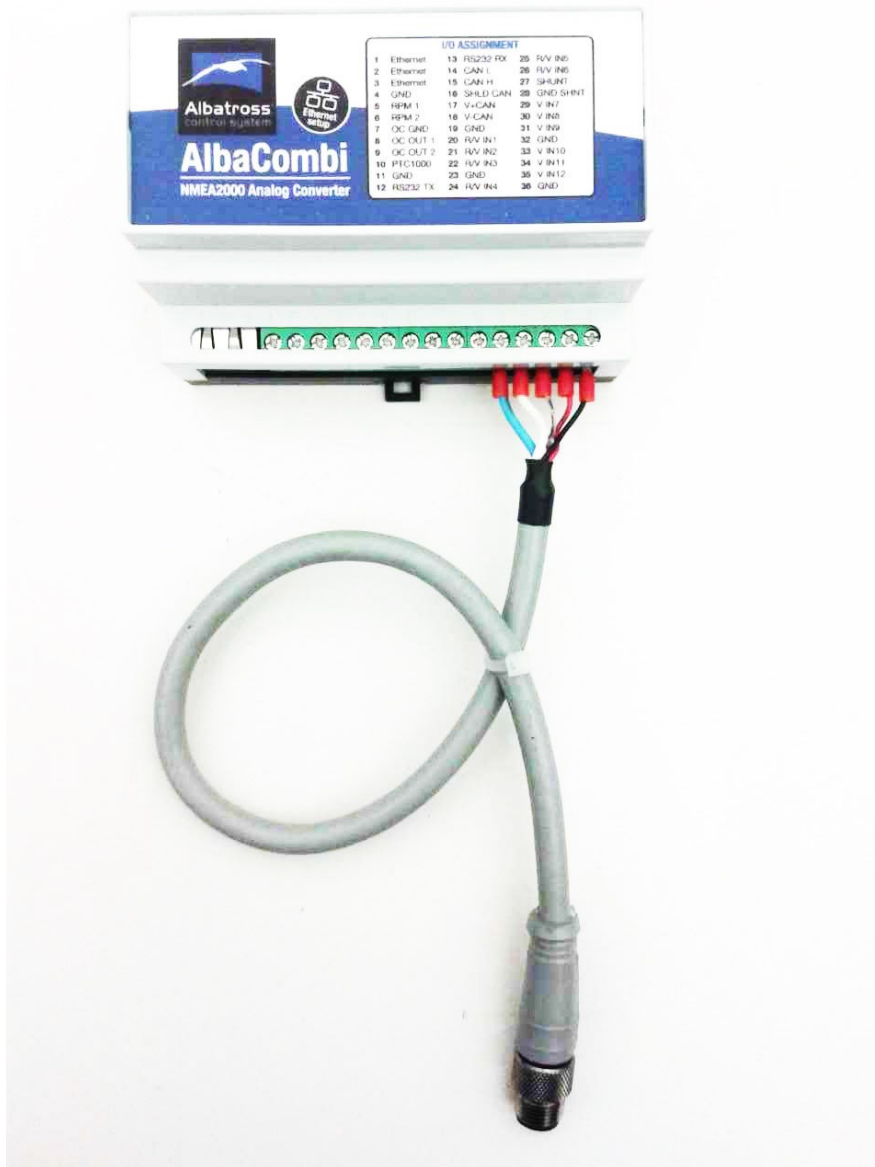
Normal connection with a NMEA2000 Spur Cable
