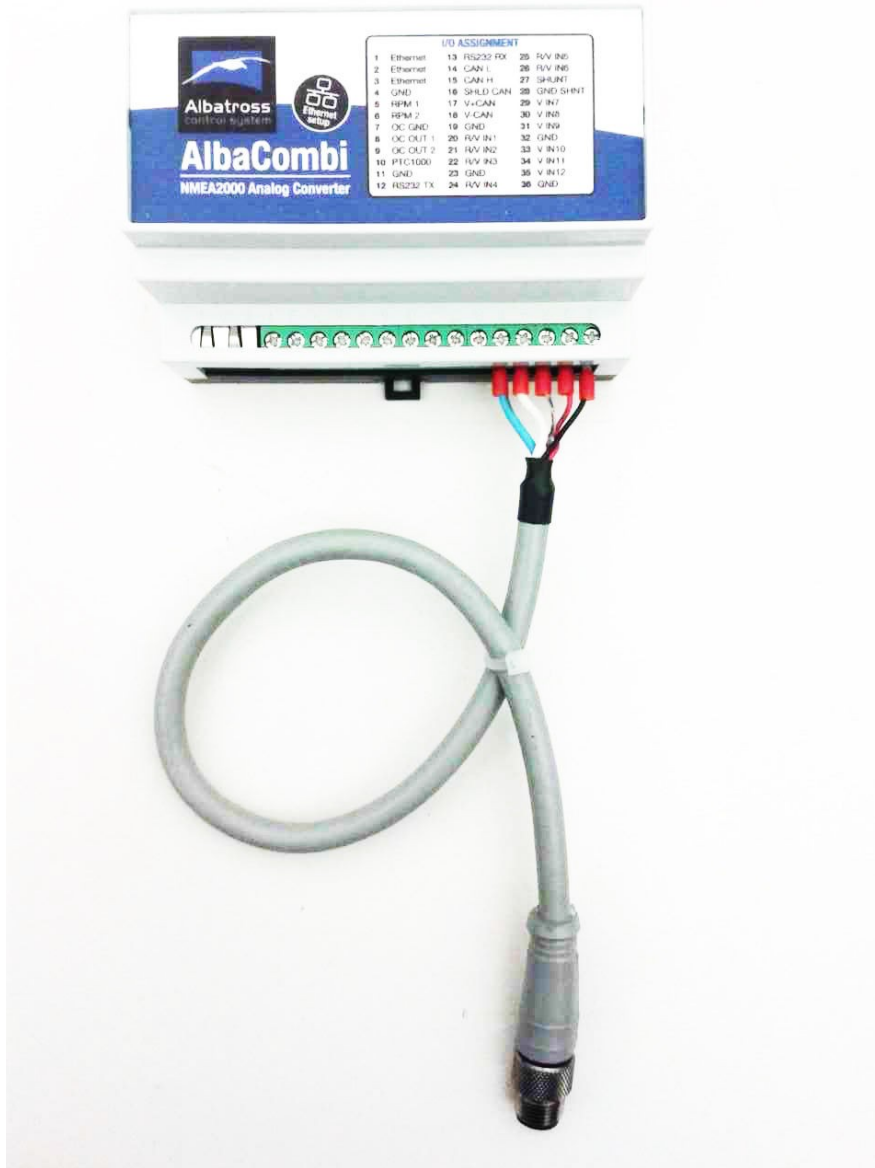
Normal connection with a NMEA2000 Spur Cable
